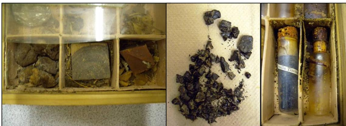
**Fig. 2.** Mechanical damage to glass and mixed materials. Fragmentation of Barbados Aloes. Leakage from phials.
