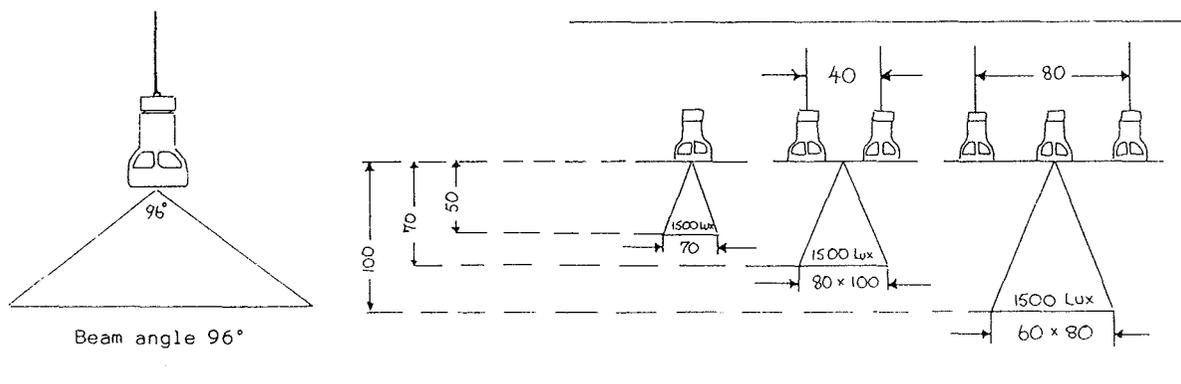
Fig. 2 Flora-Set lights, diagrammatic representation of beam angles and light intensity (measurements in cm.).
