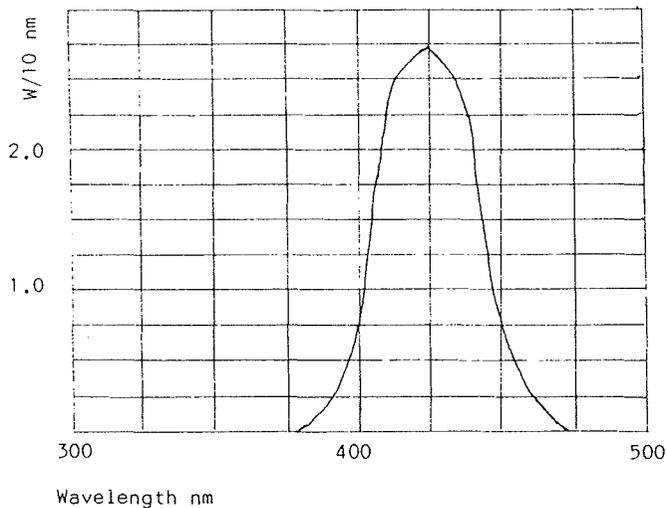
Fig. 4 Spectral analysis of actinic blue lamps.
