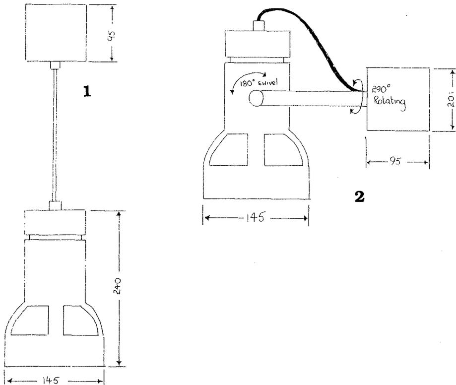
Fig. 1 Flora-Set lights, measurements in mm. 1. pendant; 2. wall-mounted.
