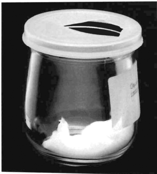
Figure 5.28 The lids of a Danish jar have a limited shelf-life and the plastic lids become brittle and split after ten to twenty years.
