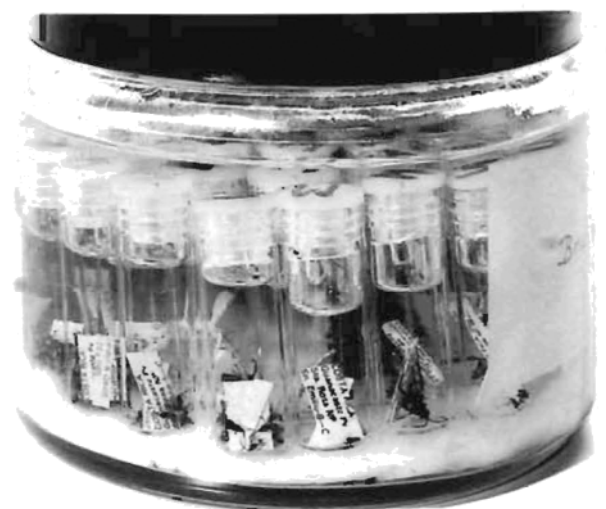
Figure 5.30 Bakelite-lidded jars with straight sides are also used for the storage of small glass vials. However, the evaporation rate is very fast and the lids have a short shelf-life of under twenty years. The Bakelite becomes brittle and, if the lid is difficult to open, it may crack or split. An improved polypropylene lid is now available to replace bakelite.
