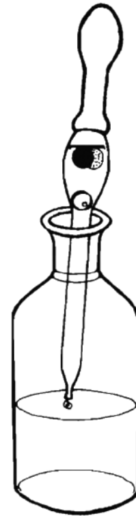
Figure 5.7 Dropper bottle with pipette reservoir containing colour-coded mapping pin heads of differing weights. The distribution of floating sunk pin heads helps to determine the nature of preservative solutions.
