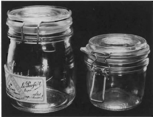
Plate 15 The LeParfait jar is the preferred choice of jar in some museums. The jar is available in a number of sizes and there is a good seal by way of a rubber gasket. The glass is sturdy, the lid cannot be separated from the jar and the sides are straight which allows for easy storage and retrieval of small glass vials (The Natural History Museum).
