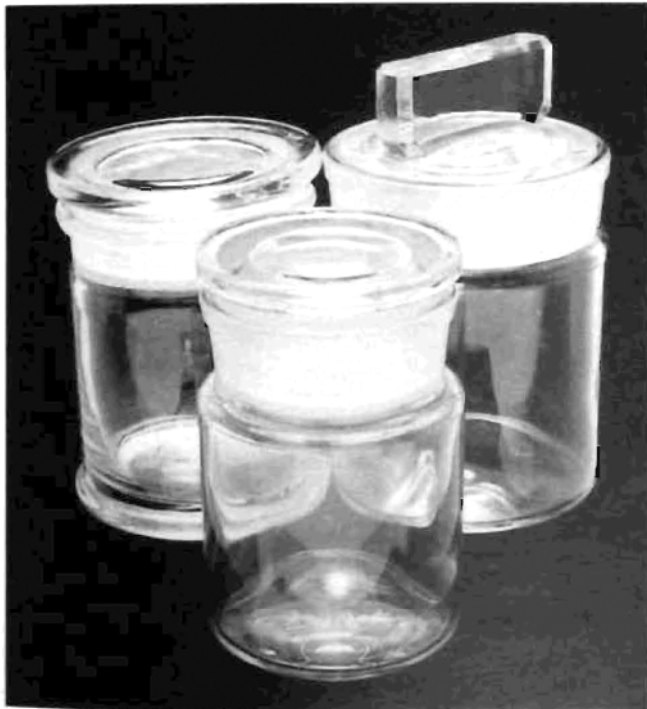
Figure 5.25 Ground glass stoppered jars are used extensively in zoological collections. The jar and stopper are made of tough borosilicate glass and manufactured in a wide range of sizes. The jar is straight-sided, allowing for easy storage and removal of specimens and the evaporation rate of the preservative is low. When 'topping up', ground glass jars should be smeared with Paraffin Soft White (BDH) around the lid and the lid rotated back into position to ensure an even and thorough seal (see text).
